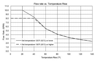
When the set temperature is 130 °F (55 °C) or higher, maximum flow rate is limited to 8.0 GPM.
